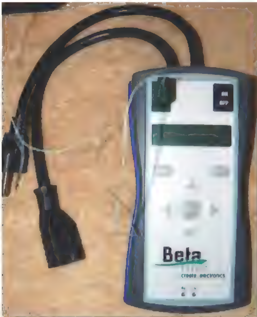
Figure 2. Beta Layout's reflow controller — US version.
